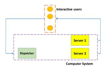
Figure 1: An interactive computer system with a dispatcher and two servers.
