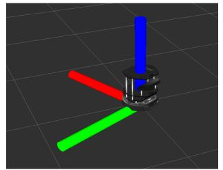
• Example: laser detected object is relative to **laser** frame. Need to transform to **map** coordinate to know where it is on the map.
