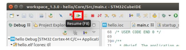
Once you notice the dev board's LED light is blinking, pause the execution by pressing the suspend key:
