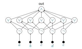
A depth-3, weft-1 Boolean circuit with inputs a, b, c, d, e.
