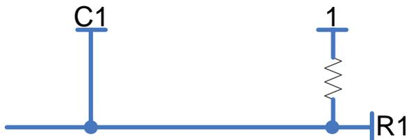
In this case, the port connected to R1 will always read the current value of C1. When C1 is Logic 0 there will be a voltage drop across the resistor, but this will not affect the value being read. Thus, the pull-up resistor accomplishes the desired task.
