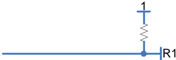
If read, the port would read a Logic 1 via the pull-up resistor.
