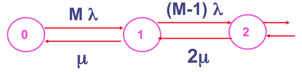
The rate of failure for one machine is  $\lambda$ . In State 0, there are M working machine, the failure rate is  $M\lambda$ .
