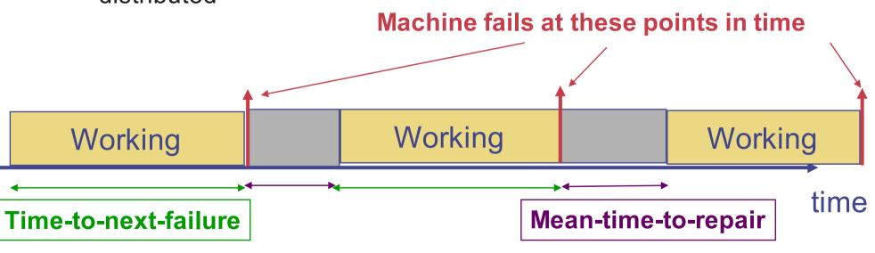
Note: Mean-time-to-repair includes waiting (or queueing) time for repair and actual time under repair
