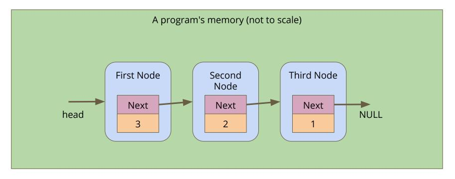
Alter the First Node's **next** to bypass the node we're removing
