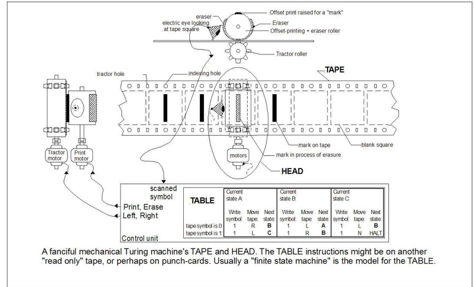
A fanciful mechanical Turing machine's TAPE and HEAD. The TABLE instructions might be on another "read only" tape, or perhaps on punch-cards. Usually a "finite state machine" is the model for the TABLE.
