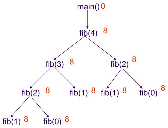
The longest weighted path is main()  $\rightarrow$  fib(4)  $\rightarrow$  fib(3)  $\rightarrow$ fib(2)  $\rightarrow$  fib(1) with the total weight of 32. So a stack space of 32 bytes is needed for this program.
