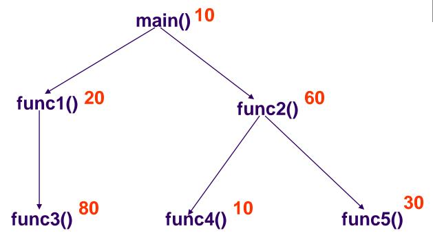
The longest path is  $main() \rightarrow func1() \rightarrow func3()$  with the total weight of 110. So the maximum stack space needed for this program is 110 bytes.
