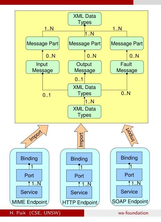
A single abstract definition is possible to be exposed to the network via a number of protocols (having different bindings, offered on different ports, etc)
