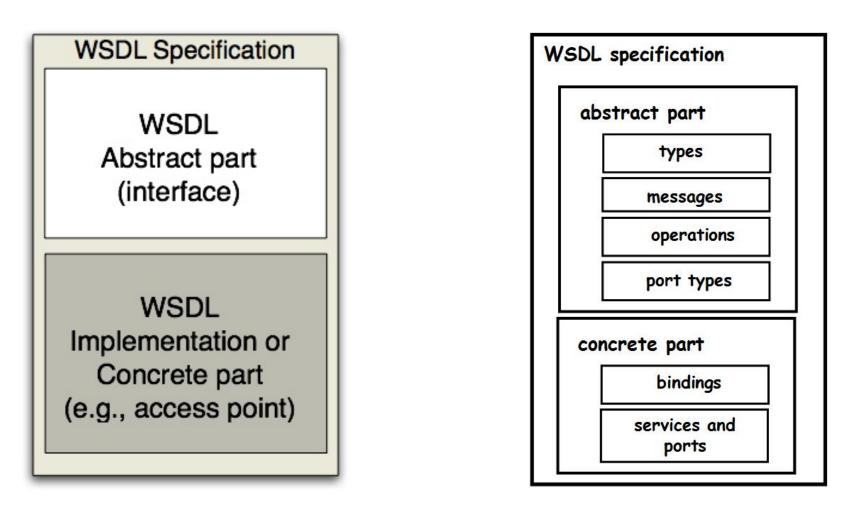
The split between abstract and concrete parts  $\rightarrow$  useful for separating Web service design and Web service deployment environment details
