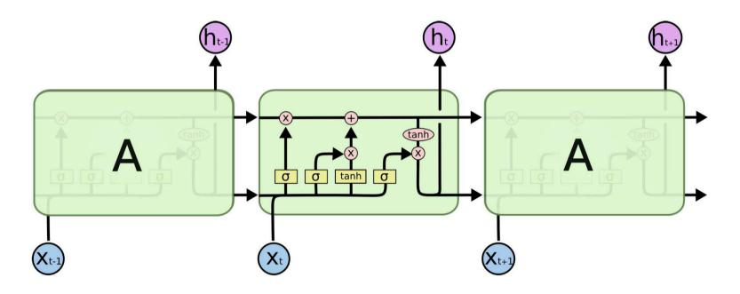
LSTM – context layer is modulated by three gating mechanisms: forget gate, input gate and output gate.
