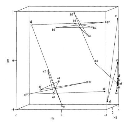
SRN with 3 hidden units can learn to predict  $a^nb^nc^n$  by counting up and down simultaneously in different directions, thus producing a star shape.
