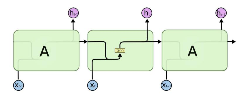
SRN – context layer is combined directly with the input to produce the next hidden layer.
