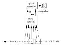
The simplest way to feed temporal input to a neural network is the "sliding window" approach, first used in the NetTalk system (Sejnowski & Rosenberg, 1987).
