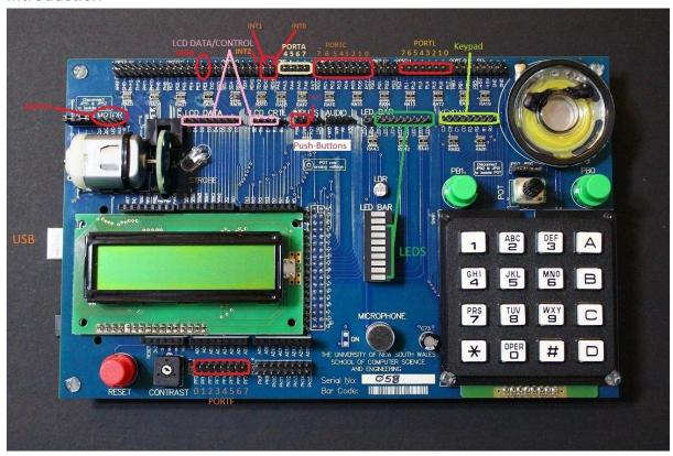
Top row and bottom rows of pins map to ATmega 2560 pins. The middle row of pins map to corresponding Input/Output devices on the board. In the top and bottom rows, 2 pins are present above each label and note that both pins are the same.
