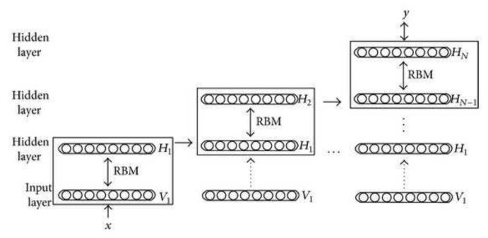
The same approach can be applied iteratively to a multi-layer network. The weights from the input to the first hidden layer are trained first. Keeping those fixed, the weights from the first to the second hidden layer are trained, and so on.
