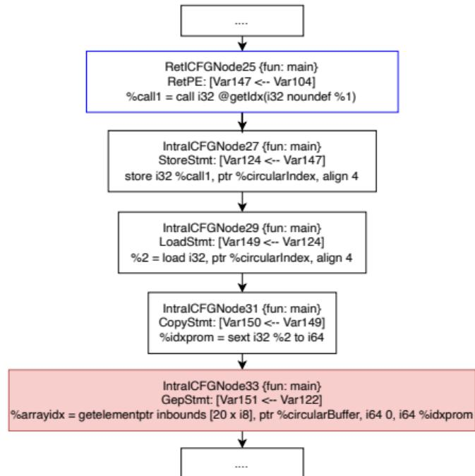
Algorithm 22: Buffer Overflow Detection for GEPSTM
