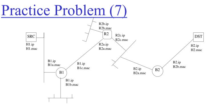
Above is a picture of a network with 2 switches (bridges) and 1 router. Each interface is labeled with an IP address and a MAC address. Imagine that host H1 is sending packet to host H2. Answer the following:
